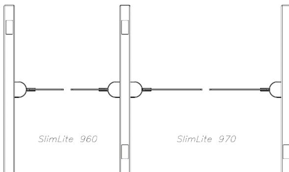
The SlimLite 960 is a modular product that can be installed as a single lane or within a multi-lane array. It can be combined with the SlimLite 970 wide lane model.
